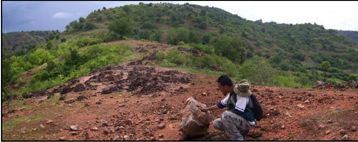
Part of the area soil sampled in the northwest part of the Kowo Prospect: Gold-anomalous, gossanous & stockwork-veined volcanic rocks crop out in foreground, and are overlain by younger post-mineral volcanic cover in background
